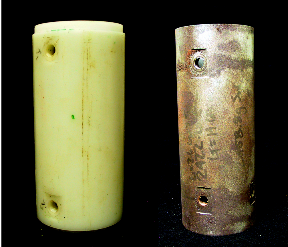
On the left is a nylon sleeve on the right is a metal sleeve.
