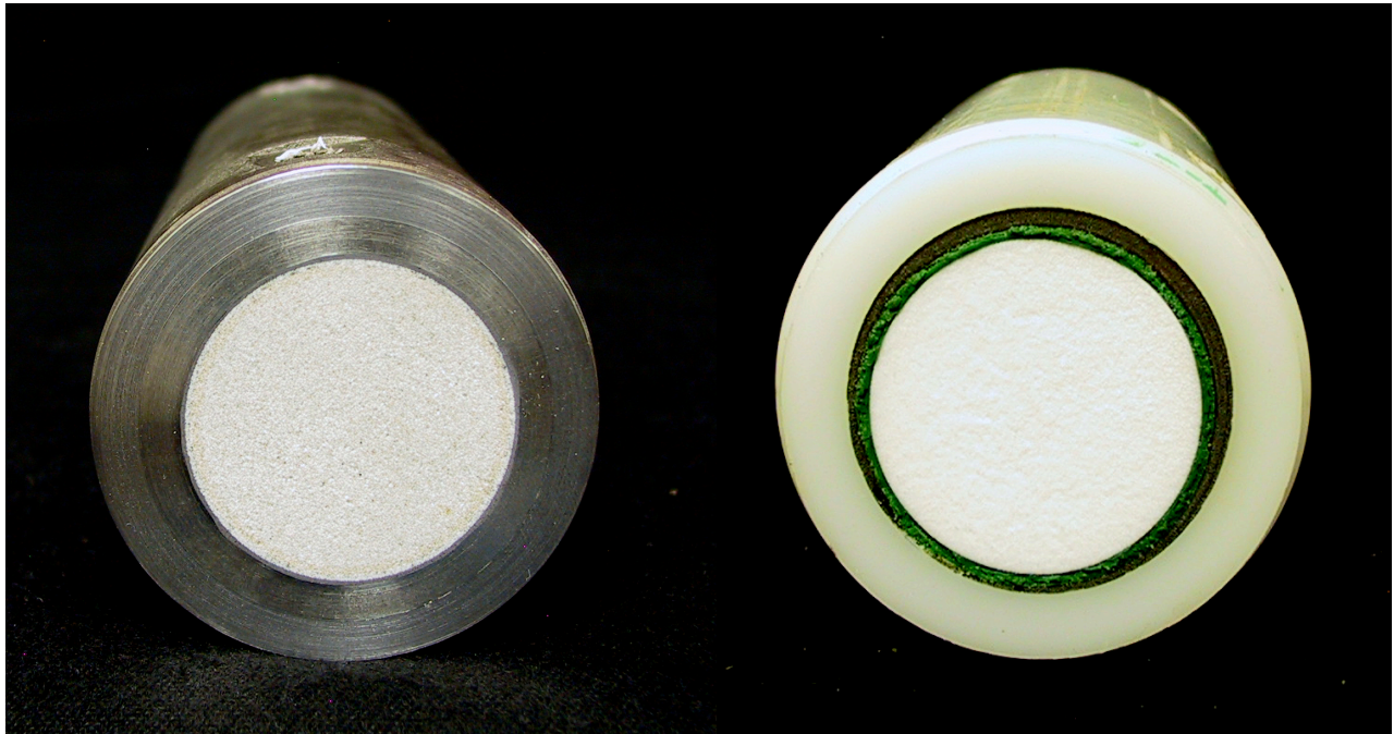
On the left is a Berea sandstone core cast in Cerrotru faced off. On right is a polyethylene core butter-coated with green Rescue Tape and cast in Sikadur 35 HiMod epoxy faced off.
