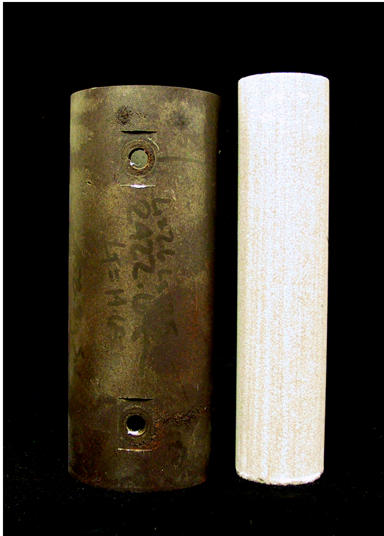
On the left is a metal sleeve and on the right is a Berea Sandstone core that is \frac{1}{4} " longer than the sleeve.
