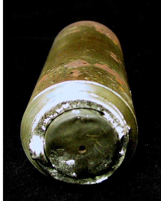
Side view and top view of a sandstone Berea core cast in Cerrotru.
