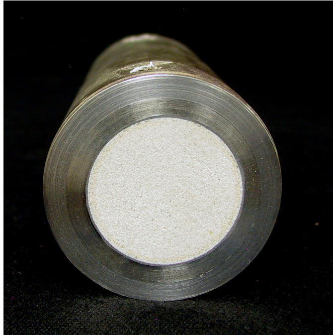
Faced-off core: picture does not contain pressure fittings, but at this stage they should be installed and the dry weight measured.
