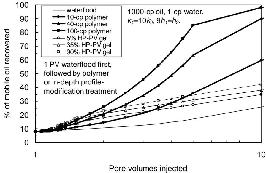
Fig. 37—Recovery with  $k_1/k_2=10$  and  $h_2/h_1=9$ . 1,000-cp oil.
