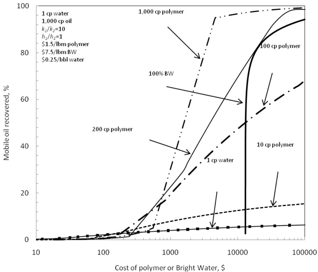
Fig. A-17—Comparison of Bright Water and polymer flooding. 1,000-cp oil,  $k_1/k_2=10$ .
