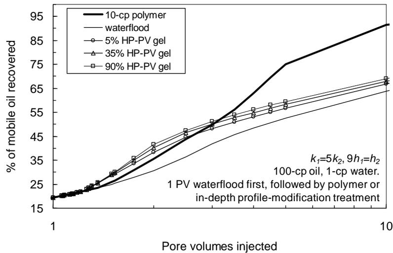
Fig. 38—Recovery with  $k_1/k_2=5$  and  $h_2/h_1=9$ . 100-cp oil.
