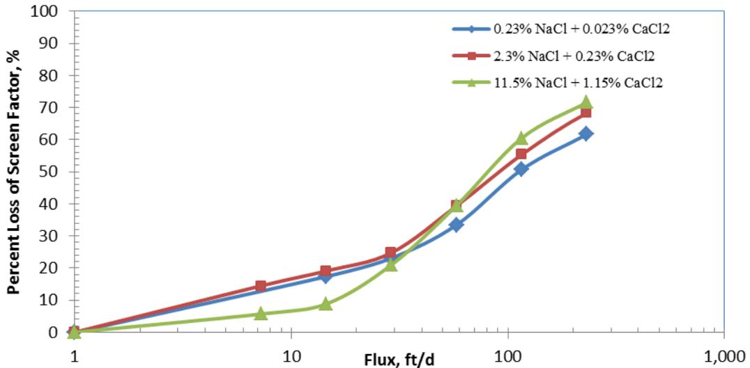
Fig. 55—Percent loss of screen factor versus flux with Ca<sup>2+</sup> present. 1000-ppm C1205.
