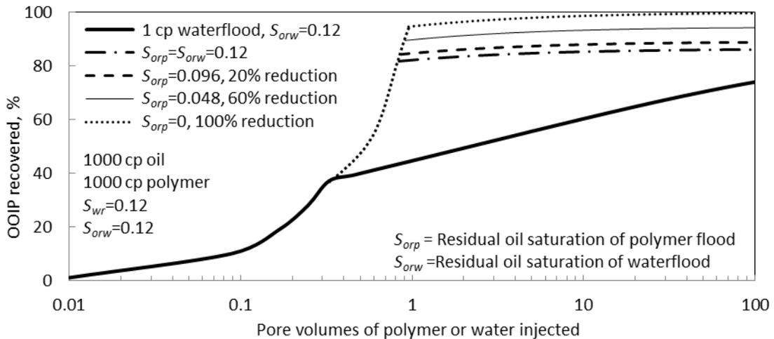
Fig. 4—1,000-cp polymer flood results for  $S_{orp}$  reduction, one layer. North Slope case.
