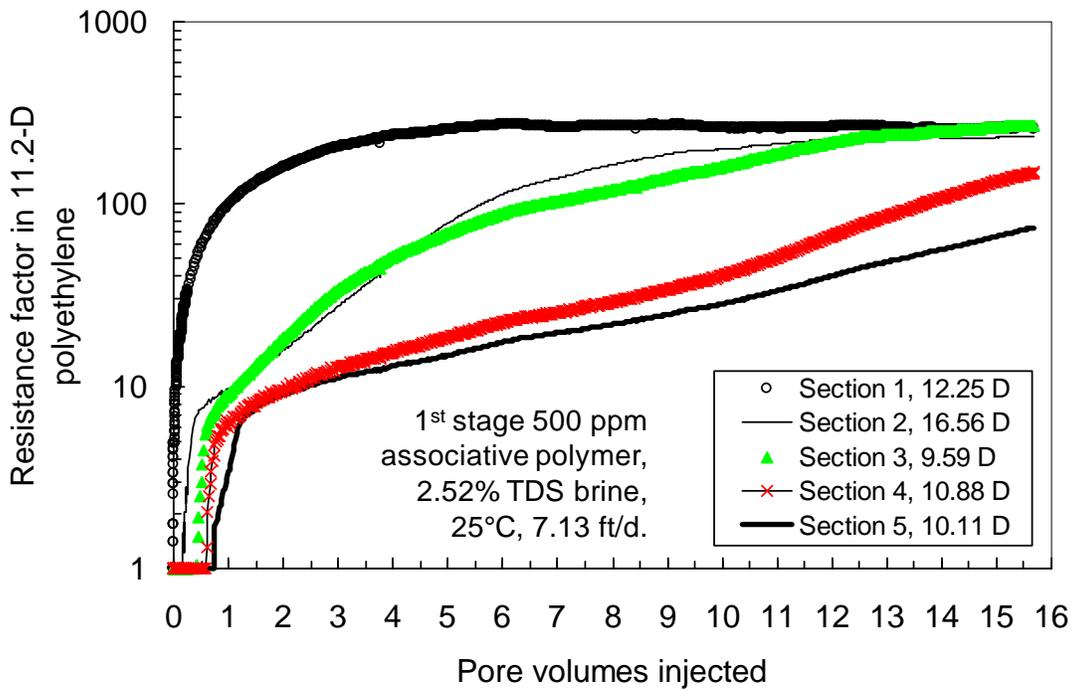
Fig. 26—Resistance factors during 1<sup>st</sup> injection of 500-ppm AP at 7.13 ft/d into 11.2-D polyethylene.
