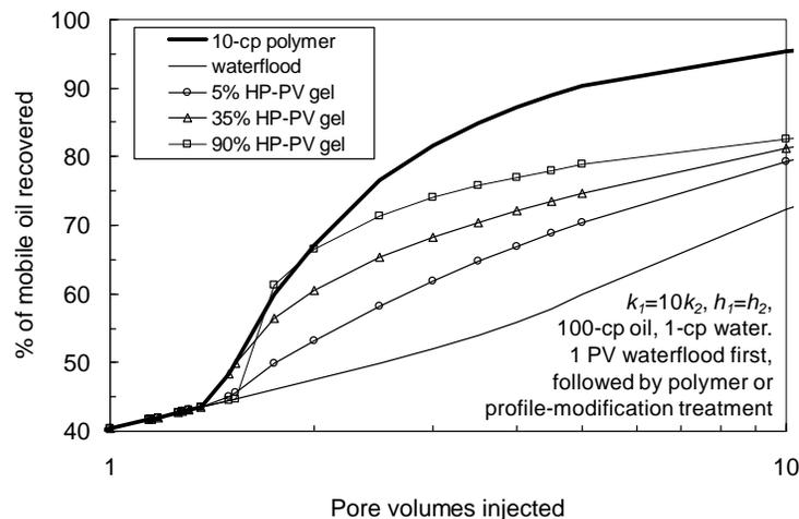
Fig. 41—Recovery with  $k_1/k_2=10$  and  $h_2/h_1=1$ . 100-cp oil.
