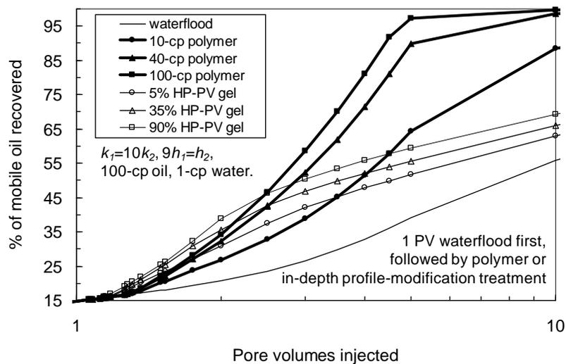
Fig. 36—Recovery with  $k_1/k_2=10$  and  $h_2/h_1=9$ . 100-cp oil.
