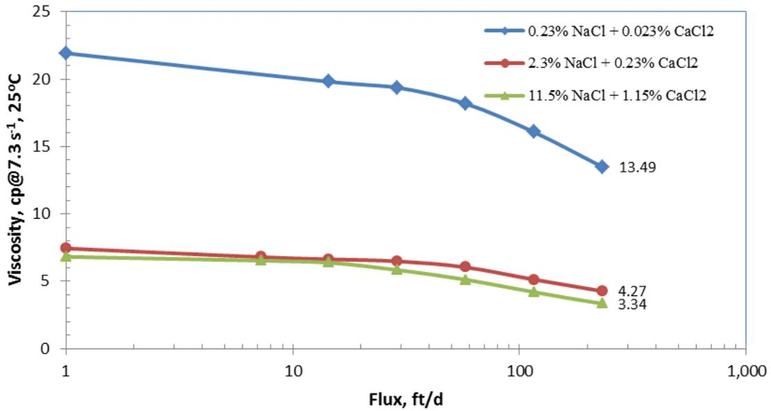
Fig. 53—Viscosity versus flux with Ca<sup>2+</sup> present. 1,000-ppm C1205.
