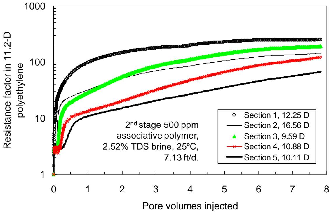
Fig. 28—Resistance factors during 2<sup>nd</sup> injection of 500-ppm AP at 7.13 ft/d into 11.2-D polyethylene.
