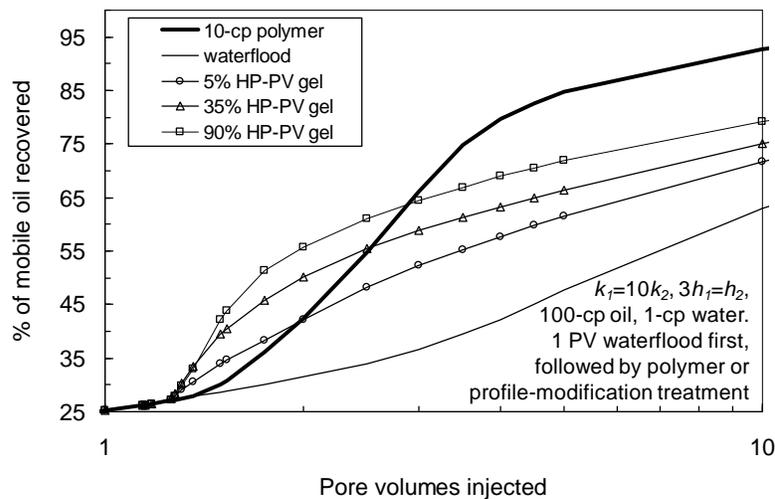
Fig. 40—Recovery with  $k_1/k_2=10$  and  $h_2/h_1=3$ . 100-cp oil.
