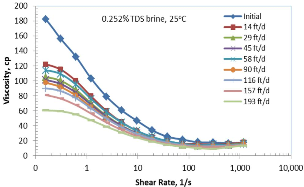
Fig. 49—Effluent viscosity versus shear rate and flux. 1,000-ppm C1205 in 0.23% NaCl, 0.022% NaHCO<sub>3</sub>.
