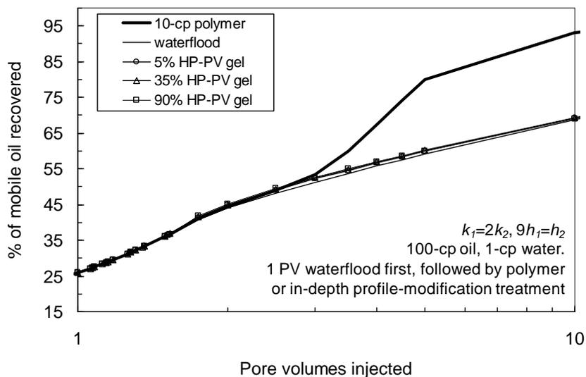
Fig. 39—Recovery with  $k_1/k_2=2$  and  $h_2/h_1=9$ . 100-cp oil.
