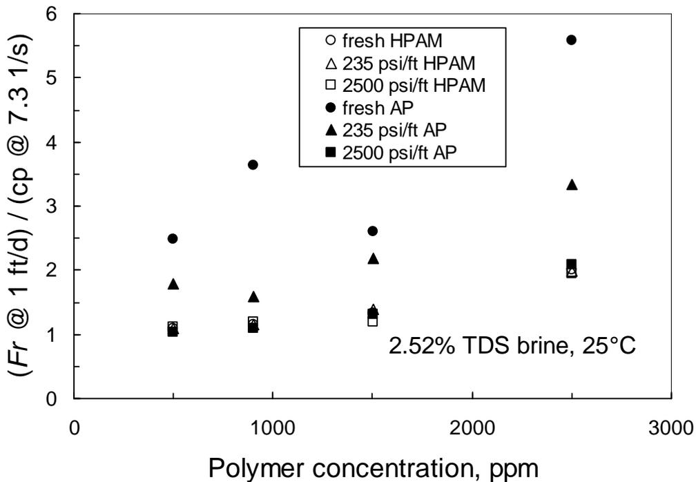
Fig. 23—Low-flux resistance factors relative to low-shear-rate viscosities.
