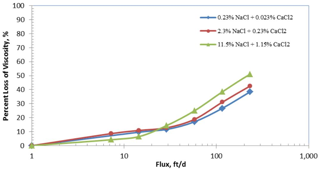
Fig. 54—Percent loss of viscosity versus flux with Ca<sup>2+</sup> present. 1,000-ppm C1205.
