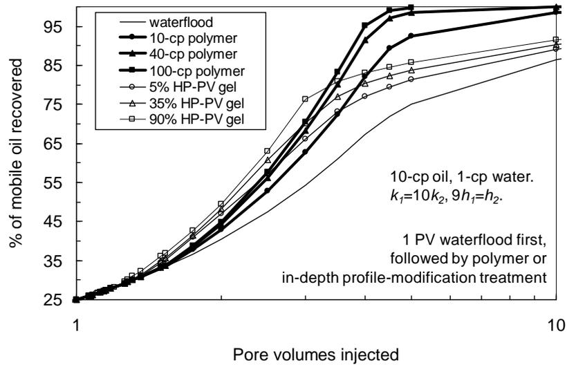
Fig. 35—Recovery with  $k_1/k_2=10$  and  $h_2/h_1=9$ . 10-cp oil.
