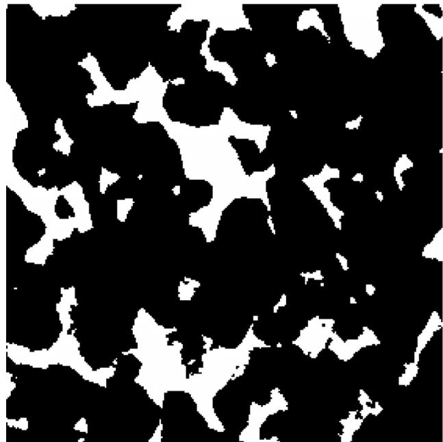
**Fig. 1—Image cross section of Berea core saturated with brine. 1.15 mm  $\times$  1.15 mm.**
