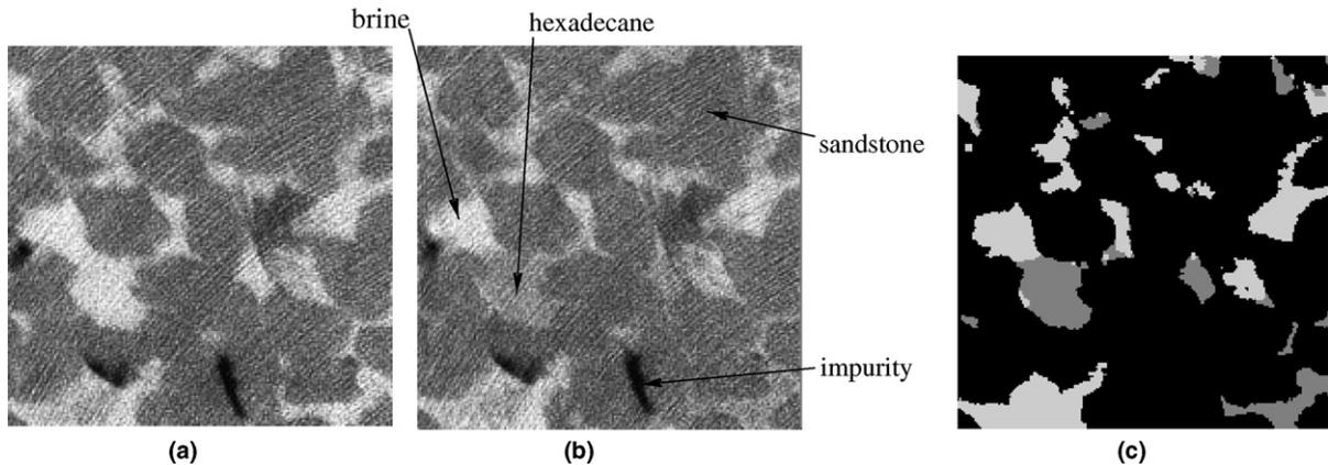
Fig. 3. (a) A subregion in  $s_w$ . (b) The same region in  $s_{or}$ . (c) Pore/rock and brine/oil segmentation results for this region.
