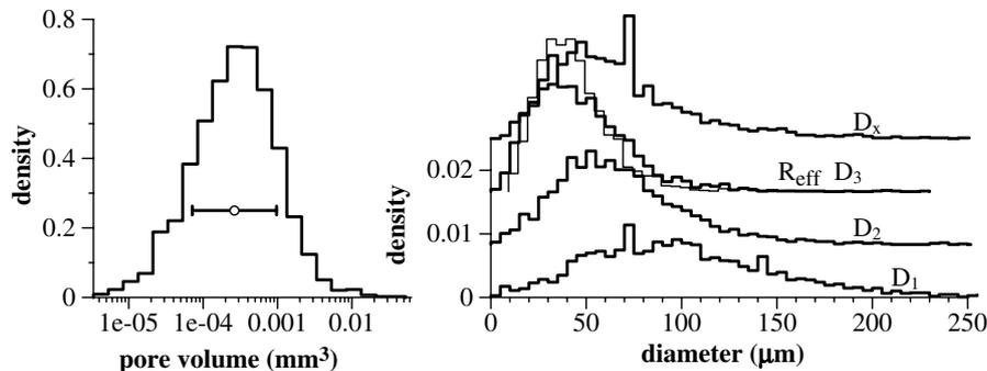
Fig. 4. (Left) Pore volume and (right) pore diameter distributions determined from  $s_w$ . (Left) The open circle and horizontal bar indicate mean and standard deviation of the distribution. (Right) All plots are to the same vertical scale, but  $D_1$ ,  $D_2$ ,  $D_3$  and  $D_x$ , have been vertically displaced from each other for visual clarity.  $R_{eff}$  (light curve) is drawn with the same vertical displacement as  $D_3$  to demonstrate the similarity between the two plots.
