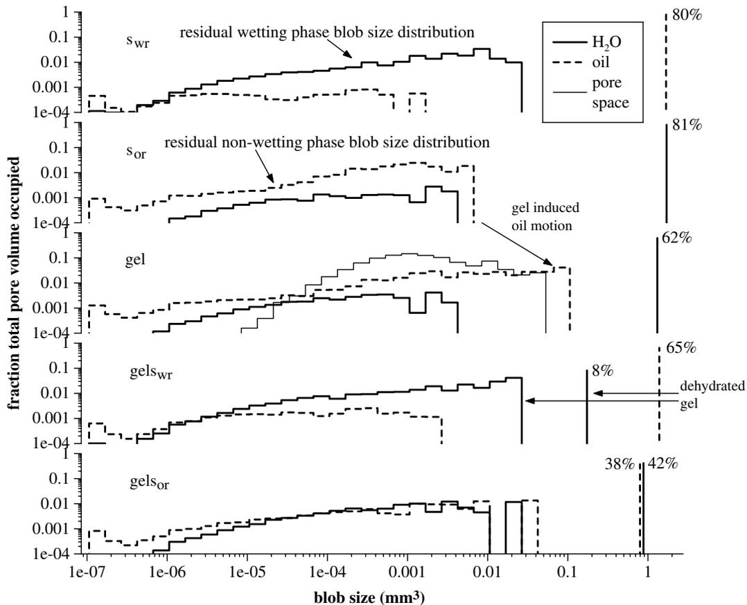
Fig. 9. Distribution of water and oil blob sizes in the images  $s_{wr}$  through  $gels_{or}$ . Blob size (x-axis) is given as a volume. The y-axis displays the total volume (expressed as a fraction of the pore volume) occupied by all blobs in each specified size range.
