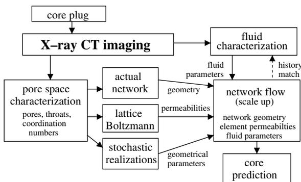
Fig. 1. A sketch of our view of the inter-relationships between XCMT, LB and NF models for improved prediction of fluid flow at core scales.
