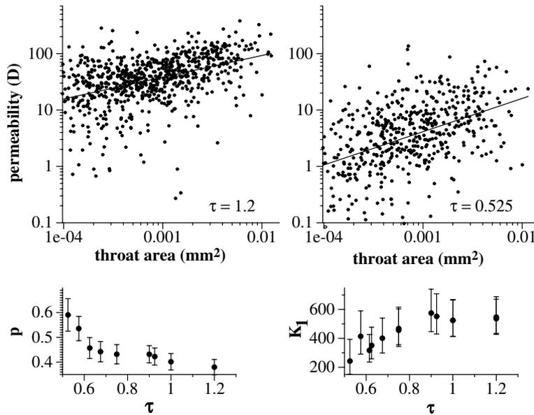
Fig. 7. (Top) LB computed throat permeabilities correlated with throat area for two values of the relaxation parameter. The straight line in each represents a least square fit. (Bottom) Dependence of the fit parameters  $p$  and  $K_1$  on the relaxation parameter.
