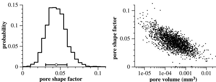
Fig. 6. (Left) Pore shape factor. The open circle and horizontal bar indicate mean and standard deviation of the distribution. (Right) Pore shape factor correlated with the pore volume. According to our definition, pore shape factor of a ball is 0.0531. The general trend of bigger pores having smaller pore shape factor leads to conclusion that bigger pores have in general more complicated, rugged surface.
