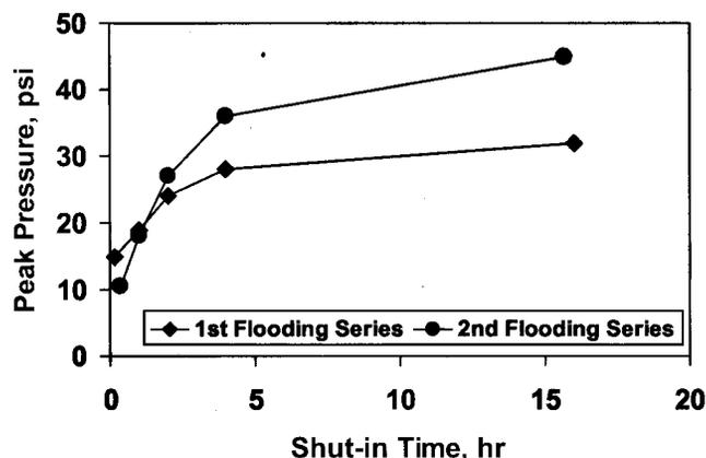
Fig. 4—Increasing peak pressure with increasing elapsed time between 8,000-cm<sup>3</sup>/hr brinefloods.
