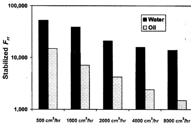
Fig. 2—Summary of variable-rate floods for the H&LMW gel in a 2-mm fracture.
