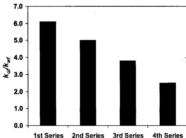
Fig. 3—Disproportionate permeability reduction as a function of brine-oilflooding series for the H&LMW gel in a 4-mm fracture.
