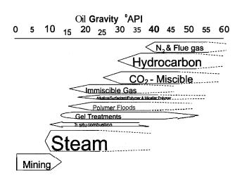
Fig. 2—Oil gravity range of oil that is most effective for EOR methods. Relative production (BID) is shown by size of type.
