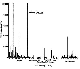
Fig. 6—EOR production vs. oil gravity outside the U.S. (data from Ref. 25).
