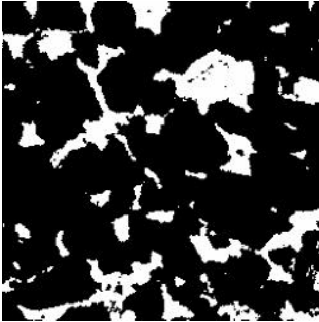
Fig. 1—XMT image cross-section of Berea. 1.15 mm x 1.15 mm.
