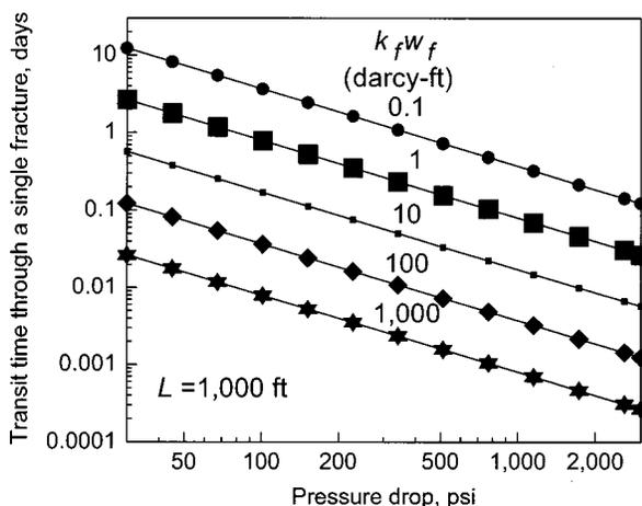
Fig. 2—Transit times through a single 1,000-ft-long fracture.
