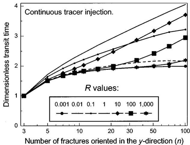
Fig. 4—Injector-producer tracer transit times in naturally fractured systems relative to that for a single direct fracture (unit-mobility displacement, fixed pressure drop, continuous injection, no dispersion); (Simulator C).
