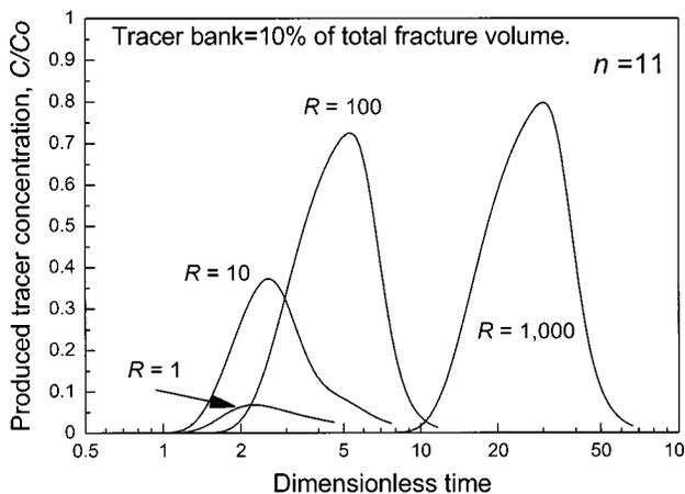
Fig. 8—Tracer curves when injector and producer were located at (1,1) and (11,2), respectively; (Simulator E).
