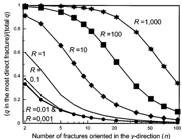
Fig. 5—Severity of channeling through the most direct  $x$ -direction fracture; (Simulator C).
