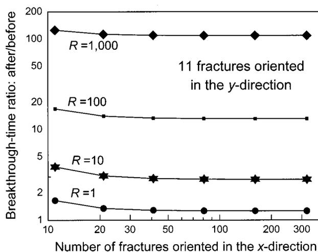
Fig. 9—Effect of plugging the most direct fracture when spacing for  $y$ -direction fractures is greater than for  $x$ -direction fractures.
