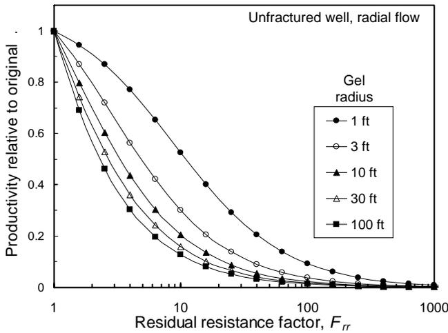
Fig. 14—Ultimate productivity after gel placement in an unfractured production well.
