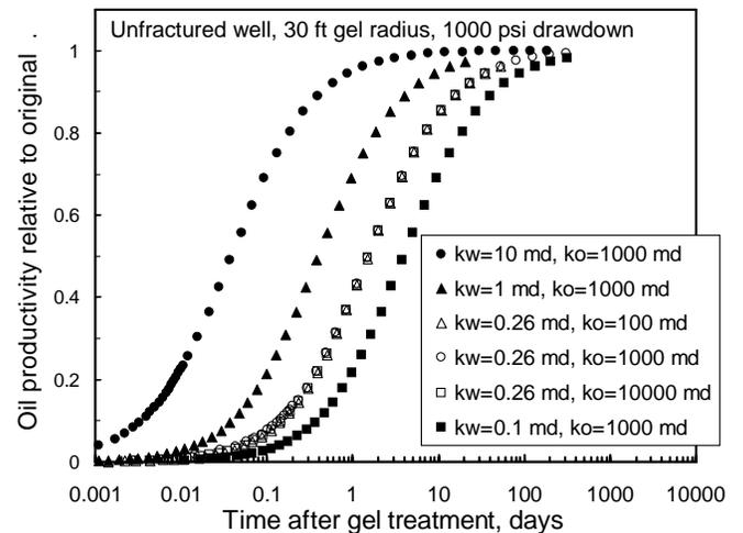
Fig. 12—Effect of  $k_w$  and  $k_o$  on oil-zone cleanup.
