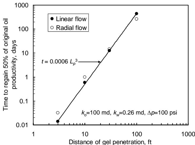
Fig. 10—Cleanup time in linear versus radial flow.
