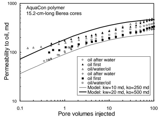
**Fig. 16—Permeability during oil injection after treatment with an adsorbing polymer.**
