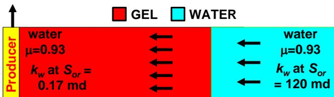
Fig. 5—Stable displacement when a water zone is returned to production after gel placement.
