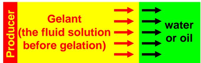
Fig. 3—Mobility ratios are usually favorable (stable displacement) during injection of gelant or polymer solutions.
