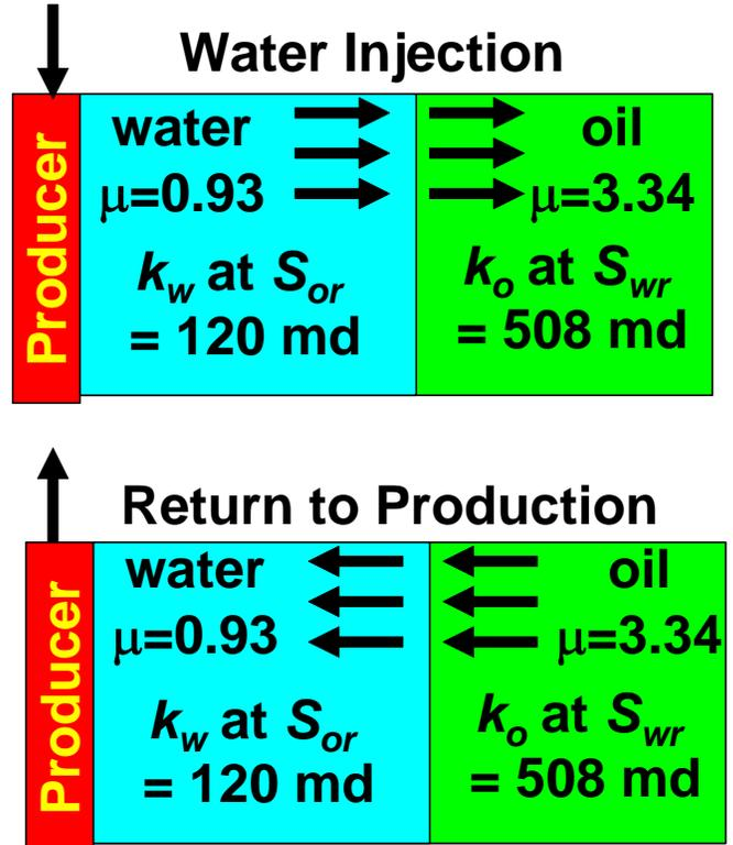
Fig. 2—Stable displacements during water injection, followed by return to production (before gel placement).
