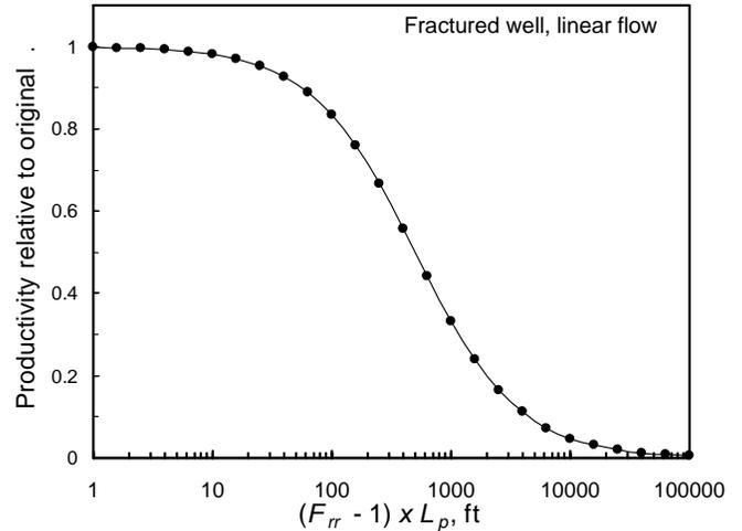
Fig. 15—Ultimate productivity after gel placement: linear flow, simplified correlation.
