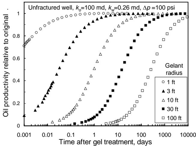
Fig. 9—Effect of radius of gel penetration in an unfractured well.
