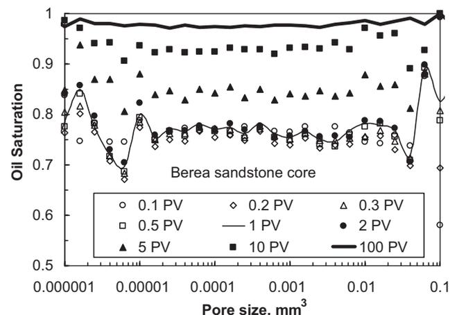
Fig. 6—Oil saturation vs. pore size and oil throughput: Berea core.
