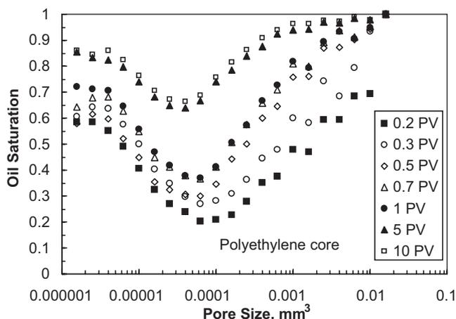
Fig. 5—Oil saturation vs. pore size and oil throughput: polyethylene core.
