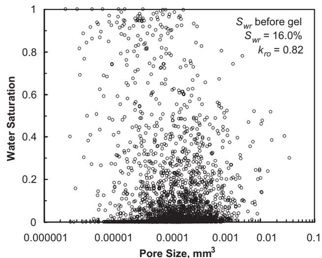
Fig. 3—Berea at  $S_{wr}$  before gel.
