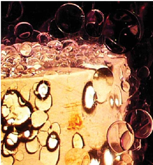
Fig. 2—Oil adhesion to the core surface during imbibition.
