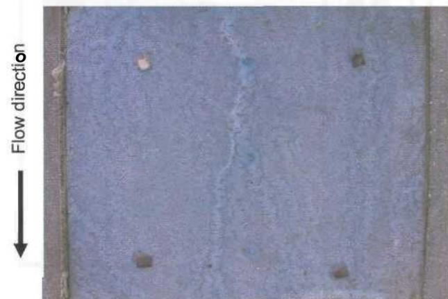
Fig. 8—Wormhole pattern for a guar-borate gel.
