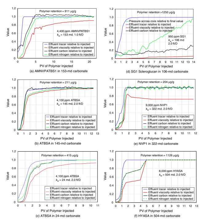
Fig. 4—Polymer-retention results at 99°C, initially saturated with injection water (6.8975% TDS) and under anaerobic conditions.
