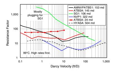
Fig. 6—Resistance factors vs. Darcy velocity for polymers in anaerobic carbonate cores at 99°C.
