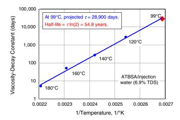
Fig. 3—Projection of decay constants at high temperatures to estimate stability at 99°C.
