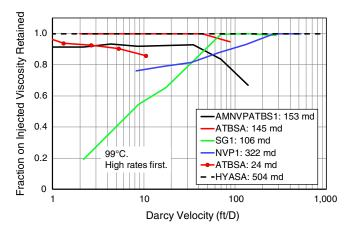
Fig. 7—Viscosity losses after injection for polymers in anaerobic carbonate cores at 99°C.
