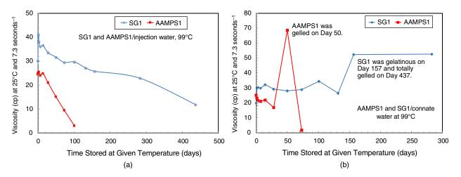
Fig. 8—Stability of AAMPS1 and SG1 at 99°C in (a) injection water and (b) connate water.
