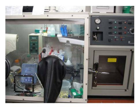
Fig. 1—Anaerobic chamber.
