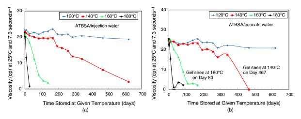
Fig. 2—Stability of ATBSA: (a) 4100 mg/L in injection water (6.9% TDS) and (b) 4200 mg/L in connate water (24.4% TDS).
