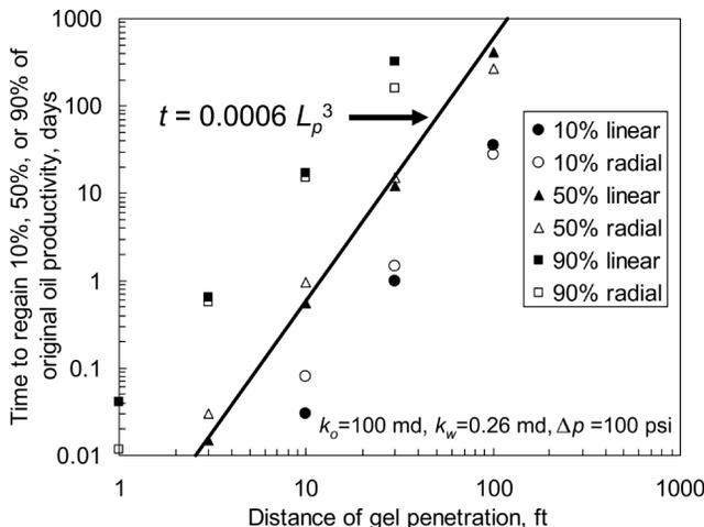
Fig. 10—Cleanup time in linear vs. radial flow.
