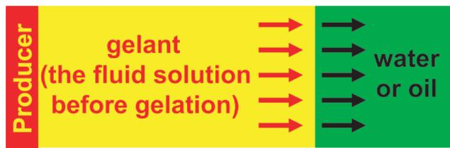
Fig. 3—Mobility ratios are usually favorable (stable displacement) during injection of gelant or polymer solutions.
