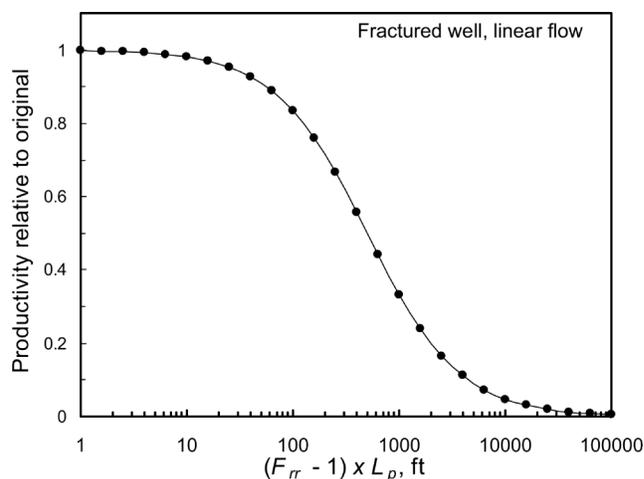
Fig. 15—Ultimate productivity after gel placement: linear flow, simplified correlation.
