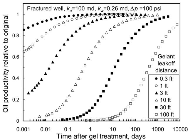
Fig. 8—Effect of distance of gel penetration from a fracture face.
