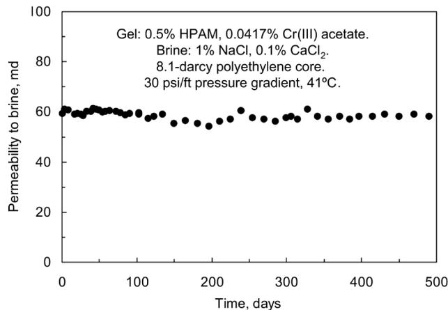
Fig. 6—Permeability to brine vs. time.
