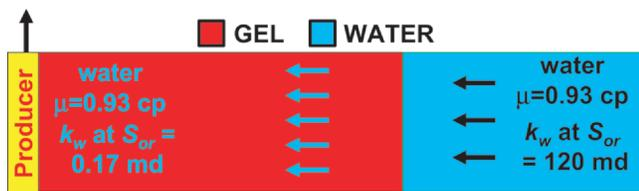
Fig. 5—Stable displacement when a water zone is returned to production after gel placement.  $M=706$ , but displacement is still stable because the entering water becomes part of the gel.
