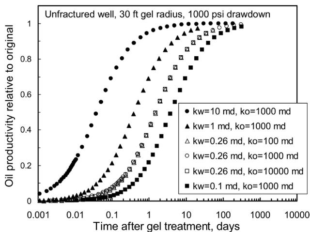
Fig. 12—Effect of  $k_w$  and  $k_o$  on oil-zone cleanup.
