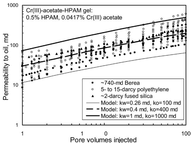
Fig. 7— $k_o$  after gel placement for many experiments.
