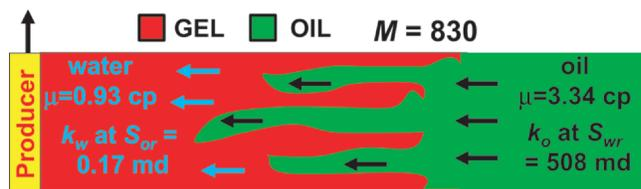
Fig. 4—Unfavorable mobility ratio when an oil zone is returned to production after gel placement.
