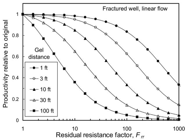
Fig. 13—Ultimate productivity after gel placement in a fractured production well.
