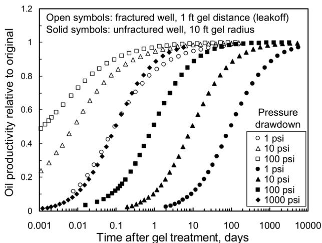
Fig. 11—Effect of pressure drawdown on oil-zone cleanup.
